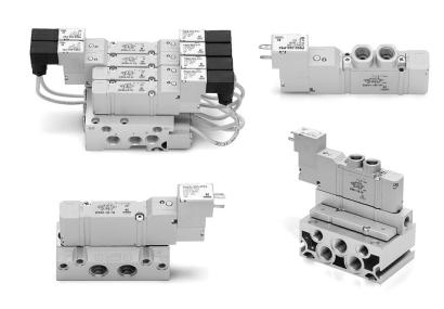
Series E valves have been designed to allow high flows with small overall dimensions. These valves are manufactured in three different sizes and are suitable for individual use or for mounting on manifolds. The manifolds allow a common inlet as well as the two exhausts and the pilot exhaust in common.
