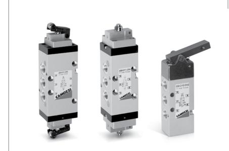
In order to facilitate the use of limit switch valves in applications where very low actuating forces and high flow rates are required, the Series 3 and Series 4 valves are equipped with new mechanical devices designed for this purpose. The Series 3 valve is designed with a mechanical lever which when operated releases an internal pilot signal to atmosphere. The sensitivity can be increased by adding a "whisker" or rod of ø 3 mm to the lever.
