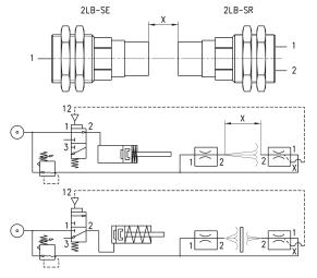
X = distance between nozzles (30 mm ÷ 80 mm)
