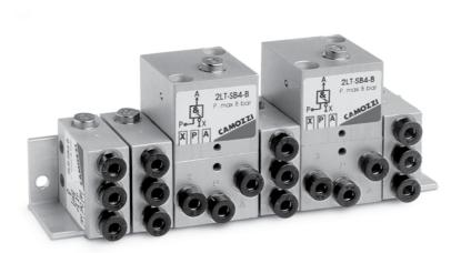
Basic logic functions Series 2L are available in 5 different models and can be mounted separately by means of 2 passing holes in the body. Bracket Mod. 2LQ-8A allows to have the inlets and outlets on the front side, facilitating the mounting of the connection tubes.
