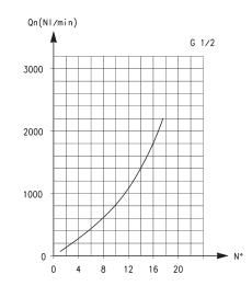
Flow Qn (Nl/min.) from  $2 \rightarrow 1$  with controller OPEN: 710 Flow Qn (Nl/min.) from  $2 \rightarrow 1$  with controller CLOSED: 410
