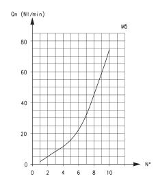
Flow Qn (Nl/min.) from  $2 \rightarrow 1$  with controller OPEN: 70 Flow Qn (Nl/min.) from  $2 \rightarrow 1$  with controller CLOSED: 33 Qn = supply pressure of 6 bar and with  $\Delta P = 1$  bar at the outlet  $N^{\circ}$  = number of screw turns.
