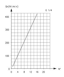
Flow Qn (Nl/min.) from  $2 \rightarrow 1$  with controller OPEN: 200 Flow Qn (Nl/min.) from  $2 \rightarrow 1$  with controller CLOSED: 70
