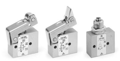
Series 2 mechanically operated miniature valves, 3/2-way normally closed, are available with M5 threaded ports or with an integrated super-rapid fitting for Ø 4mm tubes.
