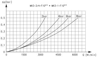
\* Reference diagram for models with filtering element = 25 µm
