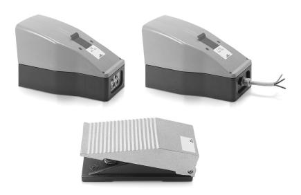
The pedals can be supplied in either a pneumatic or electrical foot operated version. The pneumatic type is available with a 5/2 valve and G1/4 front ports, which allow the fittings and silencers to be assembled conveniently on the front face. A 3/2 operation can be obtained by closing an outlet port.
