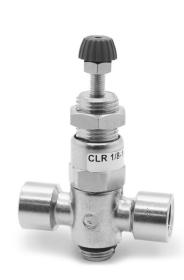
Series CLR micro pressure regulators are available with G1/8 and G1/4 connections. A piston with or without relieving and VS function (by-pass valve) has been incorporated into its design. The body is in brass, while the connection fitting is in technopolymer which guarantees maximum lightness. They can be supplied with or without banjo and can be console mounted.
