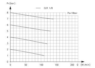
Pa = Inlet pressure (bar) Pr = Regulated pressure (bar)
