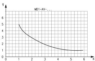
Pressurisation times as to the number of turns of the regulation screw, with downstream volume of 5 litres. A = 5 turns - B = 4 turns - C = 3 turns - D = 2 turns - E = 1 turn. K = number of turns of the regulation screw required to obtain the required pressurisation time with an inlet pressure of 6 bar. Variations of the inlet pressure can cause deviations of the pressure time by ± 20%. K = t/V where: V = volume of the downstream system in litres; t = desired pressuring time in seconds.
